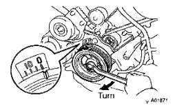
Turn the crankshaft pulley and align its groove with timing mark "0" of the No.1 timing belt cover.
