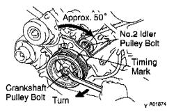
Turn the crankshaft pulley approx. 50° clockwise, and put the timing mark of the crankshaft pulley in line with the centers of the crankshaft pulley bolt and the idler pulley bolt.
