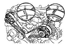
c. Check that each pulley aligns with the timing marks as shown in the illustration. If the timing marks do not align, remove the timing belt and reinstall it.
