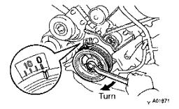
b. Slowly turn the crankshaft pulley **2 revolutions** from TDC to TDC.
