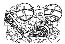
b. Check that the timing marks of the camshaft timing pulleys and timing belt rear plates aligned. If not, turn the crankshaft 1 revolution (360°).
