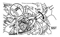
b. Using SST, turn the timing pulley. Align the installation mark on the timing belt with the timing mark of the timing pulley, and hang the timing belt on the timing pulley.
