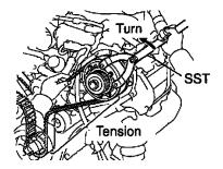
c. Using SST, turn the LH camshaft timing pulley counterclockwise until there is tension between the crankshaft timing pulley and LH camshaft timing pulley.
