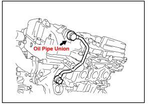
21. Remove No. 2 oil pipe union bolt from the oil pipe.
