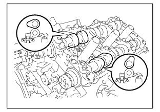
b. Uniformly loosen and remove the 8 camshaft bearing cap M6 bolts in the sequence shown in the illustration.
