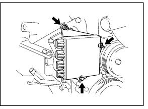
65. Install the No. 1 engine cover with the 3 clips.
