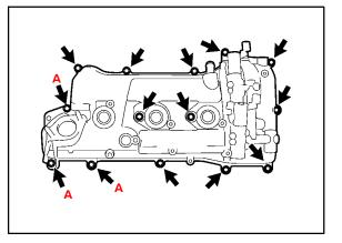
67. Install the cylinder head cover LH.
