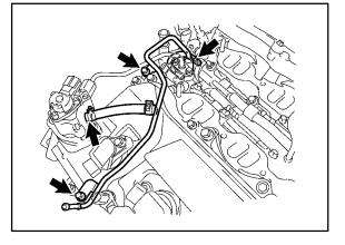
**Repair** 17. Disconnect fuel pipe No. 2.
