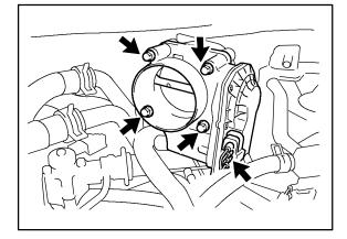
Repair 15. Remove the intake air surge
