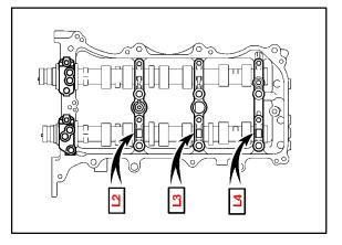
d. Tighten the 8 M6 bolts in the sequence shown in the illustration.
