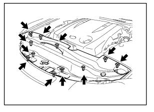
Remove the engine compartment side cover LH by removing the 5 clips.
