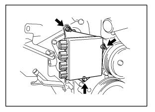
26. Remove the timing chain cover plate. Remove the 4 bolts, timing chain cover plate, and timing chain cover plate gasket.
