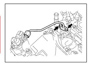
Repair<br/>Procedure<br/>(Continued)20. Remove the No. 1 oil pipe union bolt<br/>from the oil pipe.
