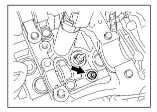
Repair 45. Install the NEW lash adjuster. Procedure
