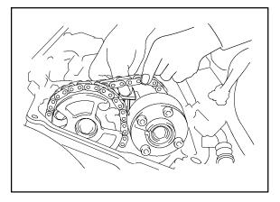
**Repair** 60. Install the camshaft bearing cap.
