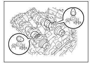
b. Uniformly loosen and remove the 9 camshaft bearing cap M6 bolts in the sequence shown in the illustration.
