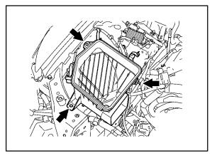
80. Install the air cleaner cap with air cleaner hose.
