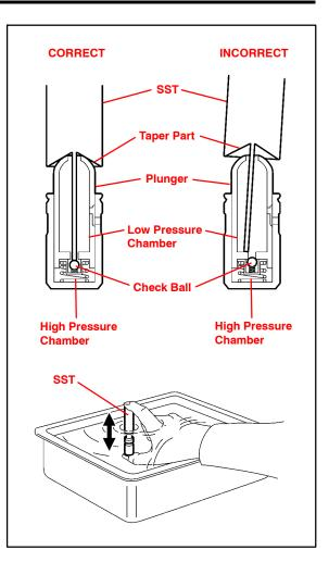
E. After bleeding the air, remove the SST. Then try to quickly and firmly press the plunger with your fingers.
