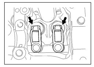
**Repair** 36. Remove the valve stem cap.
