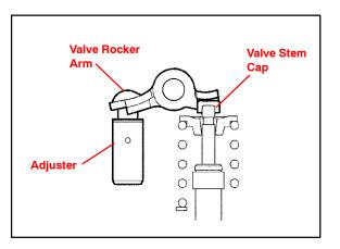
**Repair** 46. Install the NEW valve spring. **Procedure**
