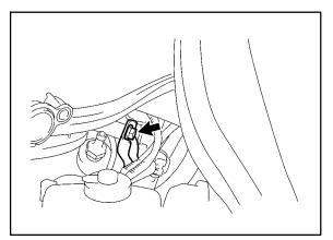
E. Connect the water hose joint with the bolt.
