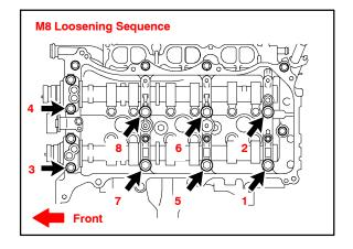
Repair 31. Remove the No. 2 camshaft.
