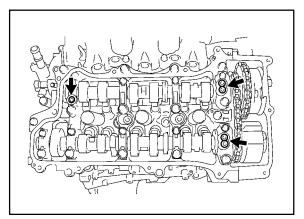
D. Install the head cover with the 14 bolts.
