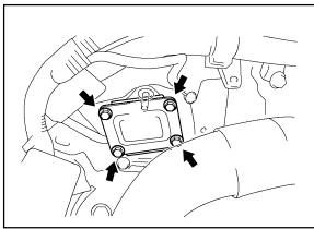
Repair<br/>Procedure<br/>(Continued)64. Install the injector driver with the bolt<br/>and 2 nuts.
