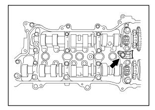
C. While holding the No. 2 chain, slide the No. 2 camshaft out toward the front of the vehicle.
