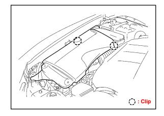
5. Remove the V-bank cover sub-assembly.
