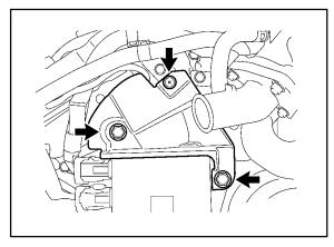
66. Install the cylinder head cover RH.
