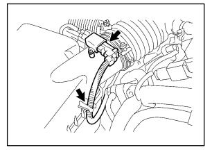
81. Connect the No. 2 ventilation hose to the cylinder head cover with the clamp.
