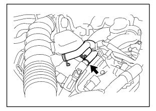
Repair<br/>Procedure<br/>(Continued)82. Install the No. 1 air cleaner inlet with<br/>the 2 bolts.
