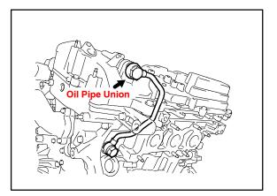
69. Install the oil pipe union bolt to the No. 1 oil pipe.
