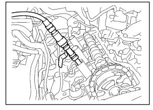
40. Pressurize the combustion chamber.
