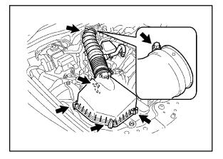
10. Remove the air cleaner case sub-assembly.
