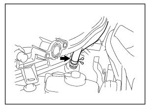
E. Remove the bolt and water hose joint from the intake air surge tank.
