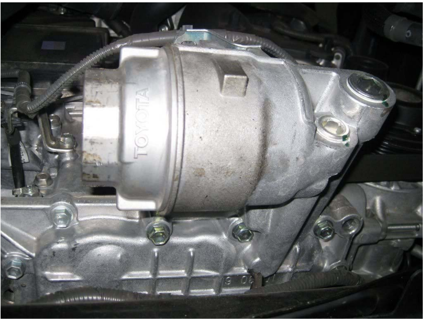
8. Follow the instructions on the filter box to remove the old filter. I had two oil filter wrenches that would have worked. Neither was the official Toyota SST which costs an arm and a leg.
