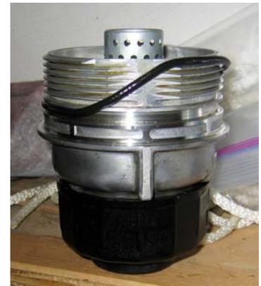
new small "O" ring positioned in groove
