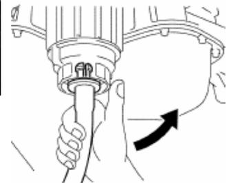
Once the oil stops running out, remove the adapter by twisting it to one side at the hose, then pull it out and set it aside (see illustration).
