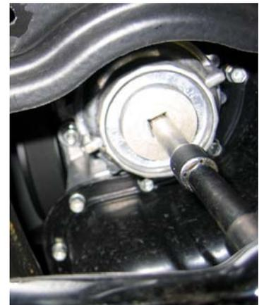
If the "O" ring is not in place, some oil will spill during the next step (draining the filter housing).
