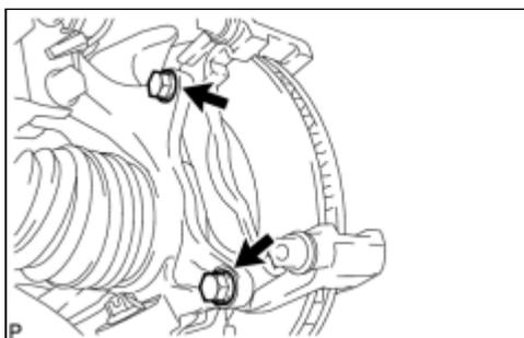
(a) Install the front disc brake cylinder mounting to the steering knuckle with the 2 bolts.
