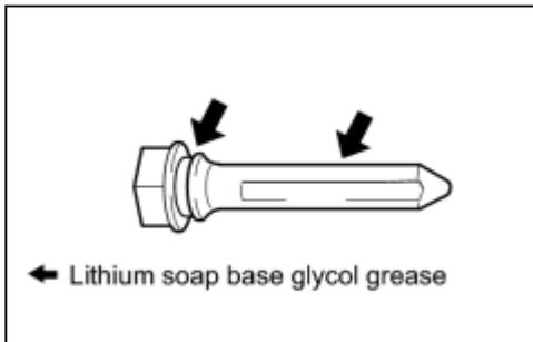
(a) Apply the lithium soap base glycol grease to the sliding part and the seal surface of the No. 1 front disc brake cylinder slide pin.
