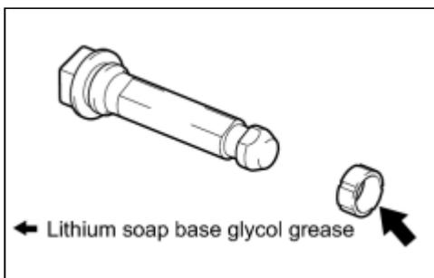
(a) Apply lithium soap base glycol grease to a new front disc brake cylinder slide bushing.
