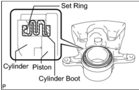
(a) Install the cylinder boot to the disc brake cylinder assembly.
