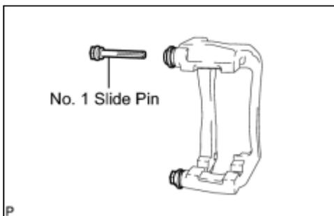
(b) Install the No. 1 front disc brake cylinder slide pin.
