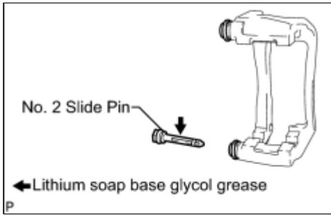
(b) Install the No. 2 front disc brake cylinder slide pin to the bottom side of the front disc brake cylinder mounting.
