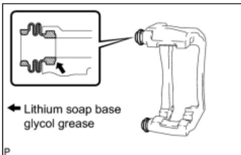
(a) Apply lithium soap base glycol grease to the seal surface of 2 new front disc brake bushing dust boots.
